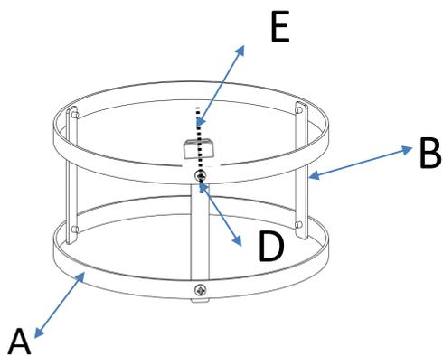
Connect the 3pcs support piece(B) and the 2 rings(A) with the screws(D) and nuts (E)
